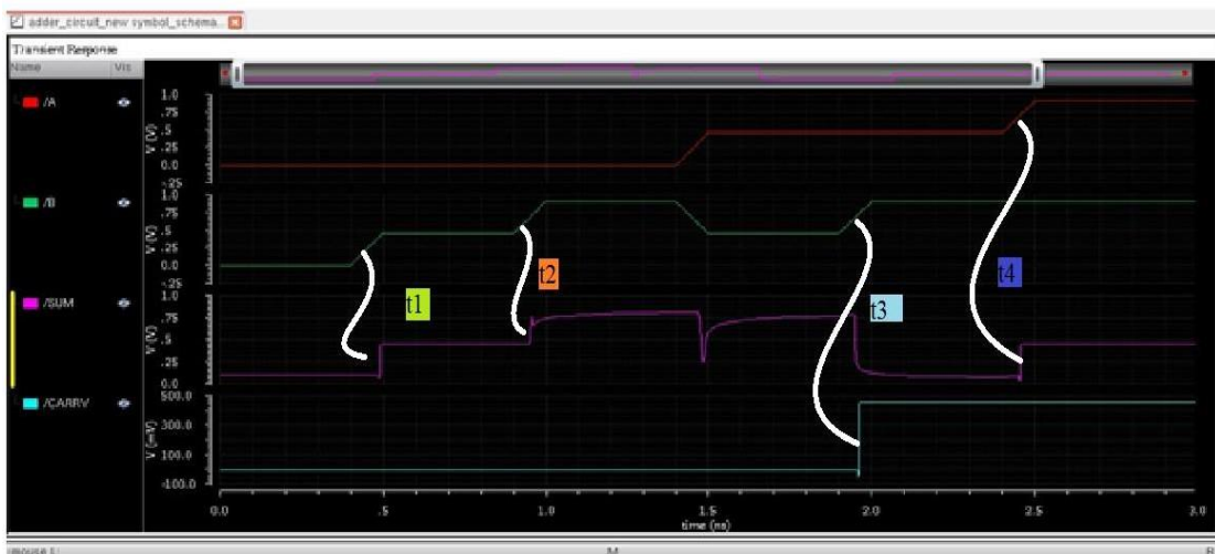
Fig.5.3 Waveform for delay calculation of proposed Half adder
