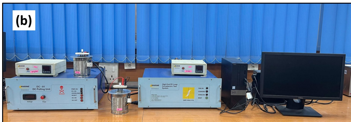
Figure 2.11: (b) PE loop tracer from Marine India available at CFMRL, Department of Applied Physics, Delhi Technological University, Delhi.
