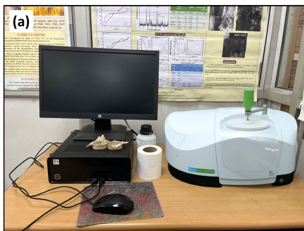
Figure 2.8: (a) FTIR setup facility present at CFMRL, Department of Applied Physics, Delhi Technological University, Delhi.
