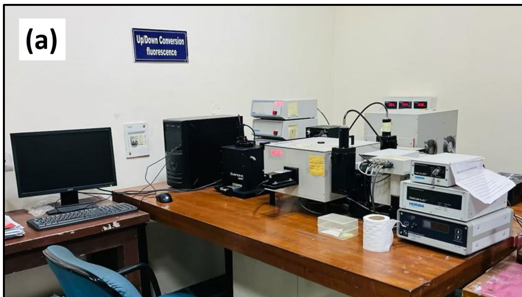
Figure 2.10: (a) Upconversion luminescence spectroscopy using 980 nm laser present at USIC, Delhi University, Delhi.
