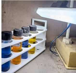
Figure 3.3. Photocatalytic dye degradation
