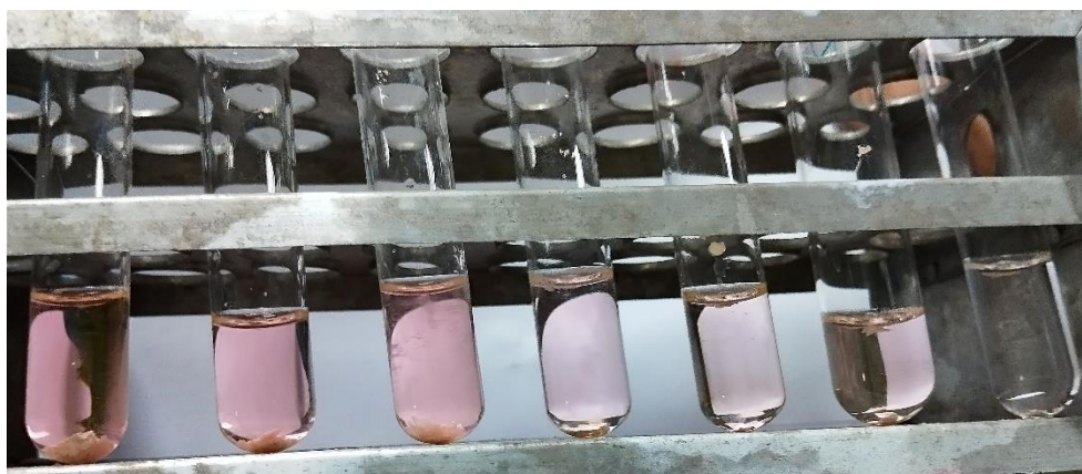
Fig. 8 Illustration showing the degradation of eosin dye with ZnNPs.
