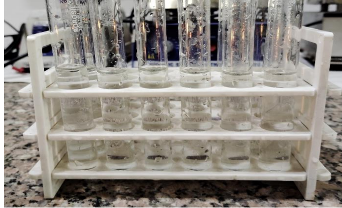
Fig. 3.1 Serial dilution test tubes consisting of a sequence of Dilutions ranging from 10^{-1} to 10^{-10} .
