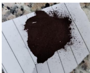
Fig. 3.7 Dried powder of rust obtained after drying in a Hot air oven for 2h.
