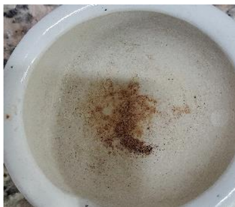
Fig. 4.2 Powder of Iron oxide nanoparticles obtained after drying in a Hot air oven for 2h.
