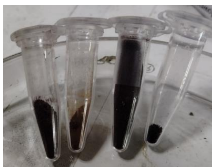
Fig. 4.3 Manufacturing of IONPs by rust and utilizing the bacterial supernatant for reducing the metal ion.
