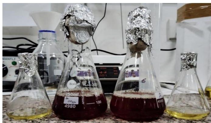
Fig. 3.8 Conical flask containing (a) Control containing only supernatant, (b) and (c) supernatant of two different bacteria containing rust, (d) Control containing supernatant of another bacterial strain
