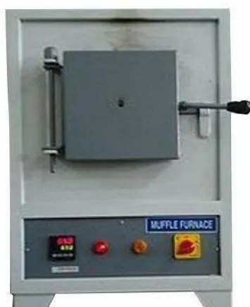
Fig 3.1.2:- Furnace used for sintering
