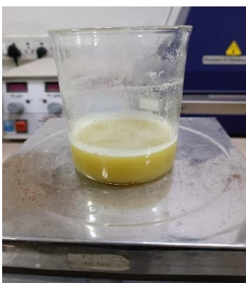
Fig. 3.9 An observable alteration in the color of the solution occurs upon the addition of NaOH to maintain a pH level of 12.
