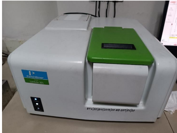
Fig.3.12 Analysis of ZnO nanoparticles using PerkinElmer UV/Vis Lamda 365.
