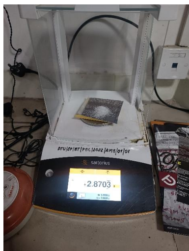
Fig. 3.7 100mM zinc sulfate heptahydrate weighed and added in 100 ml Distilled water.
