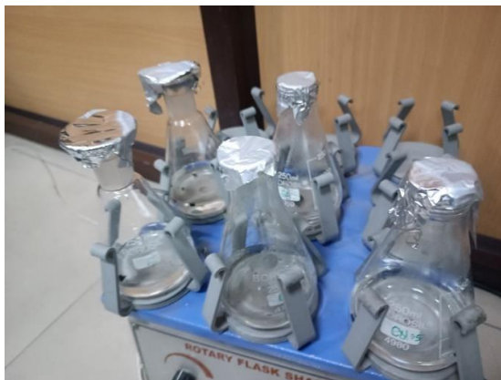
Fig. 3.14 Heavy metal (Cd) solution of 500 PPM containing different concentrations of biochar placed on a Rotary Flask Shaker at 100 rpm.
