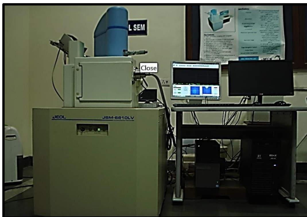
Figure 2.4 Photograph of JEOL Japan Mode: JSM 6610LV SEM
