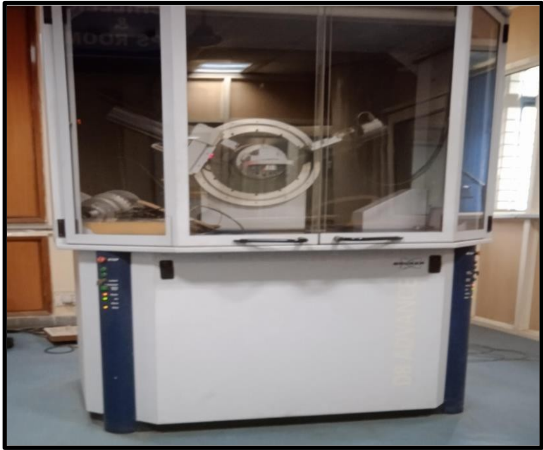
Figure 2.3 Cu-K \alpha radiation, \lambda= 1.5406 \text{ \AA} , Make Bruker, Model: D8 Discover
