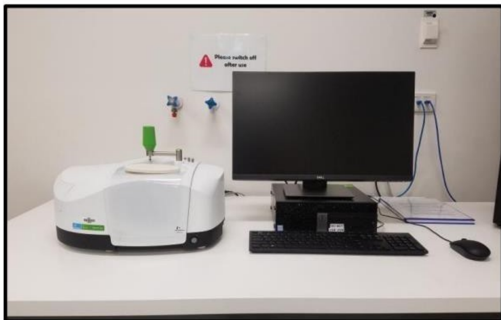
Figure 2.5 Photograph of Perkin Elmer Two-Spectrum FTIR spectrometers
