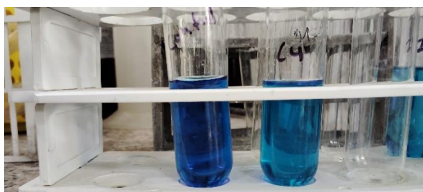
(A) Photocatalytic degradation action of copper NP on MB dye after 60 min under sunlight.
