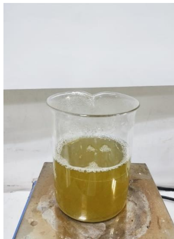
Fig. 3.6 Copper sulphate pentahydrate solution with plant extract after water bath @70°C.
