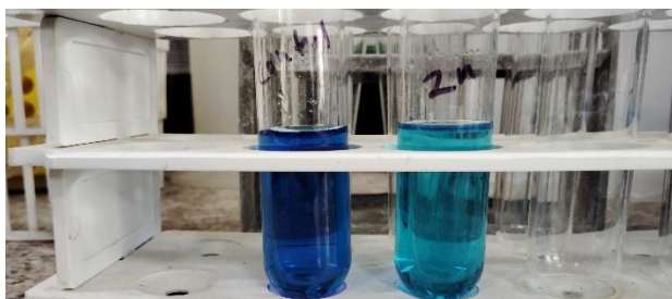
(B) Photocatalytic degradation action of zinc oxide NP on MB dye after 60 min under sunlight.
