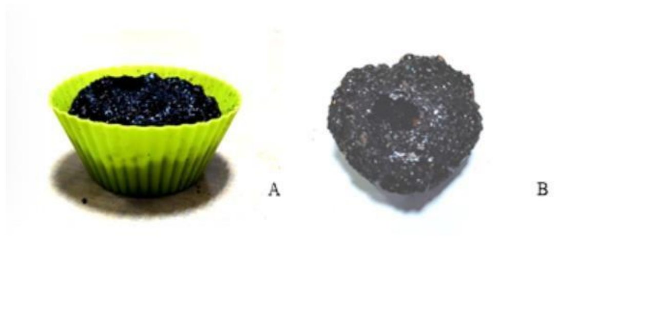
Fig.5.3: Glucose based non-isocyanate polyurethane (“A” in the Mold, “B” without it).
