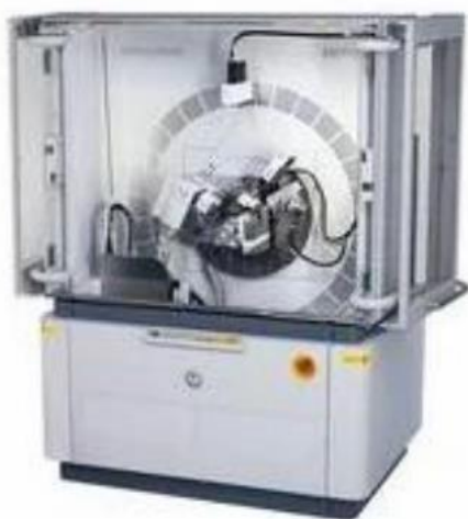
Fig 4.2: Powder X-Ray Diffraction (PXRD), utilizing a high-resolution Bruker diffractometer
