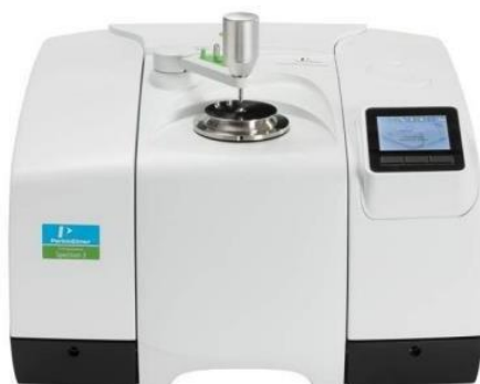
Fig.4.1- Perkin Elmer Frontier ATR-FTIR provided by an ATR Miracle diamond crystal.
