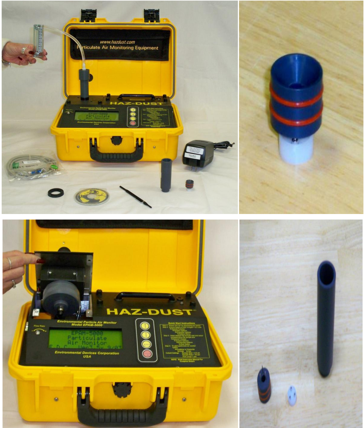
Figure 3.3: Instrument used in present study. a) Picture of EPAM-5000. b) Picture of impactor jet. c) Picture of sensor lid. d) Picture of impactor jet, impactor cup and impactor sleeve. (Clockwise).
