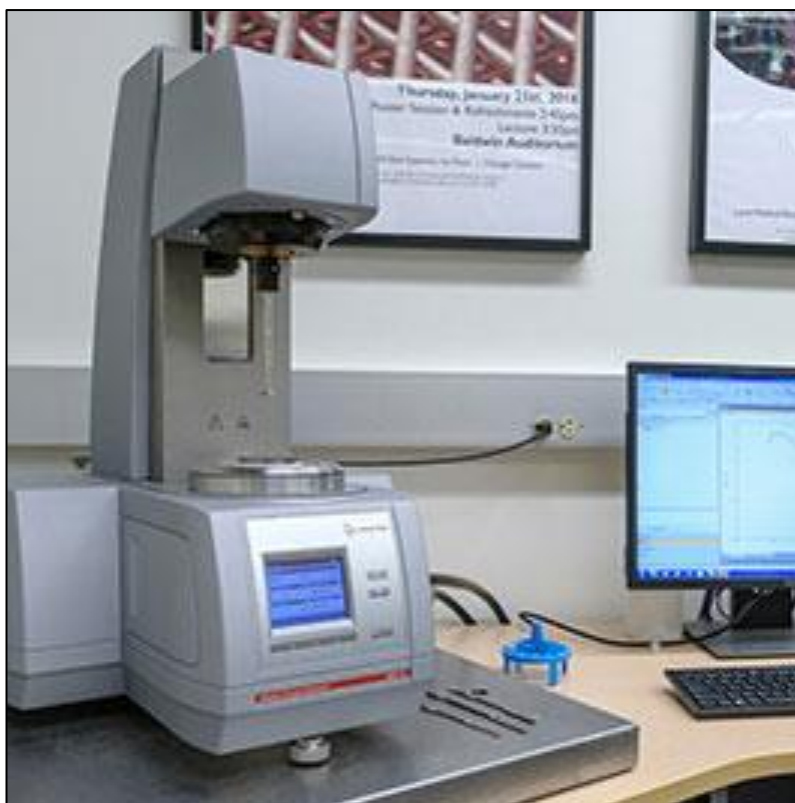
Figure 2.11. Photograph of the Anton Paar MCR 302 rheometer used in the study.
