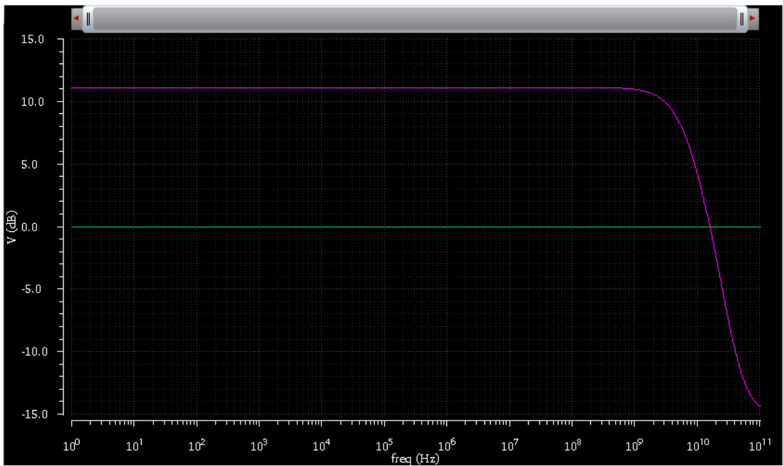
Fig 4.7.2 Proposed LNA gain at 1.5V
