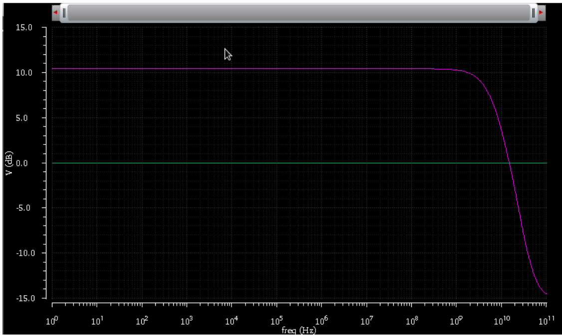
Fig 4.4.2 Proposed LNA gain at 1.2V
