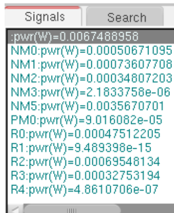
Fig 4.9.2 Proposed LNA power consumed at 1.5V
