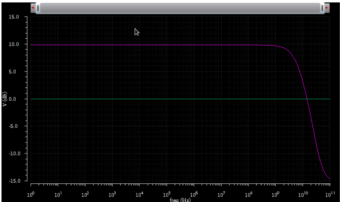
Fig 4.1.2 Proposed LNA gain at 1V
