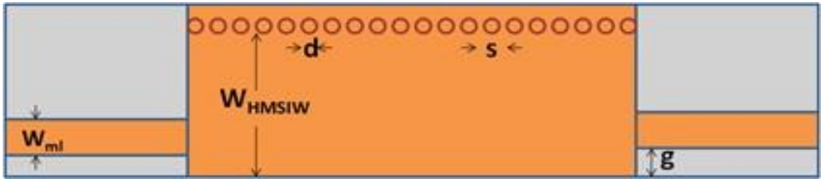
Figure 7.1. Geometrical configuration of the top of HMSIW ( W_{ml} = 1.5 , W_{HMSIW} = 7 , d = 0.4 and s = 0.8 ; all in mm)
