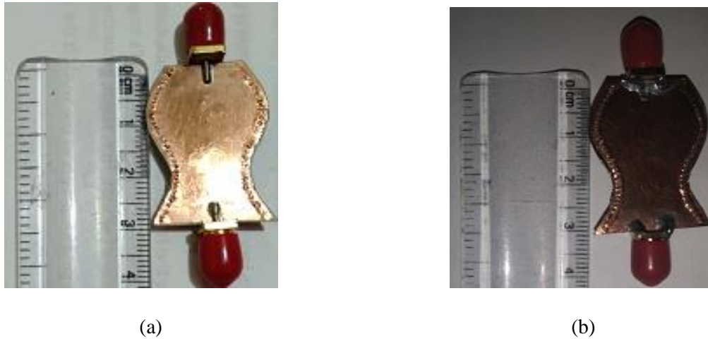
Figure 3.6 Fabricated SIW (a) Top View (b) Back View
