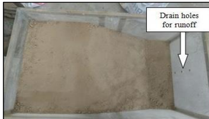
Fig. 3. 2: Frame-type box model with soil slope
