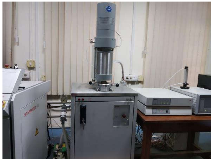
Fig. 3.12. Thermal mechanical analyzer (TMA Q400 V7.4)
