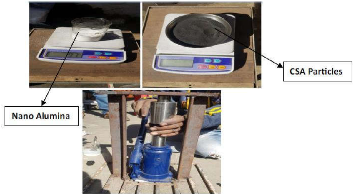
Fig. 3.5. Creating a powder using pure aluminium and nano-alumina
