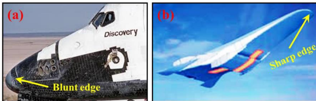
Figure 1.3 (a) Represent the digital image of a space shuttle orbiter with blunt edge [13] (b) Indicate sharp leading edge of hypersonic Vehicle [14].
