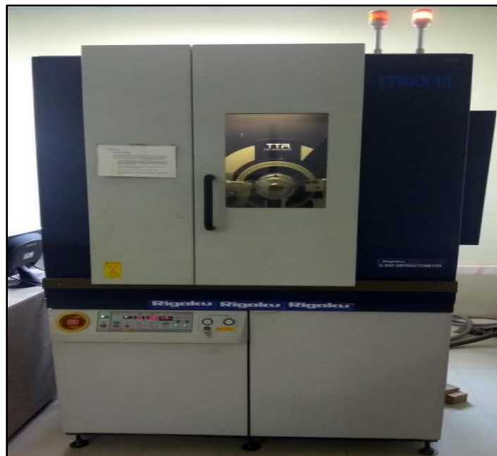
Figure: 3.7 X-ray diffractometer (Rigaku, Japan (Model: TTRAX III) used in the study
