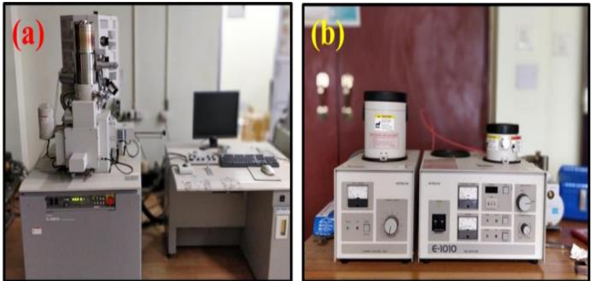
Figure:3.8 (a) the digital image of field emission scanning electron microscope (FE-SEM) supplied by Hitachi, Japan (Model: S-4800) and (b) is the digital image of ion sputtering unit (Hitachi, Model: E-1010, Japan) used to coat the samples before FE-SEM.
