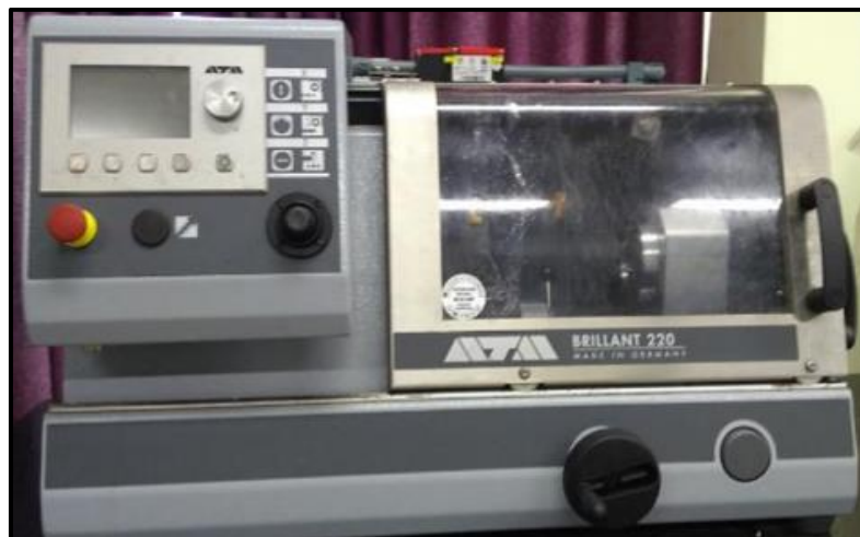
Figure 3.3: High speed Diamond saw (ATM Brilliant 220) used for cutting the samples.
