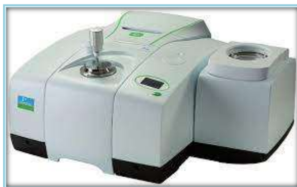
Fig. 2. 4: Perkin Elmer's frontier FT-IR spectrometer
