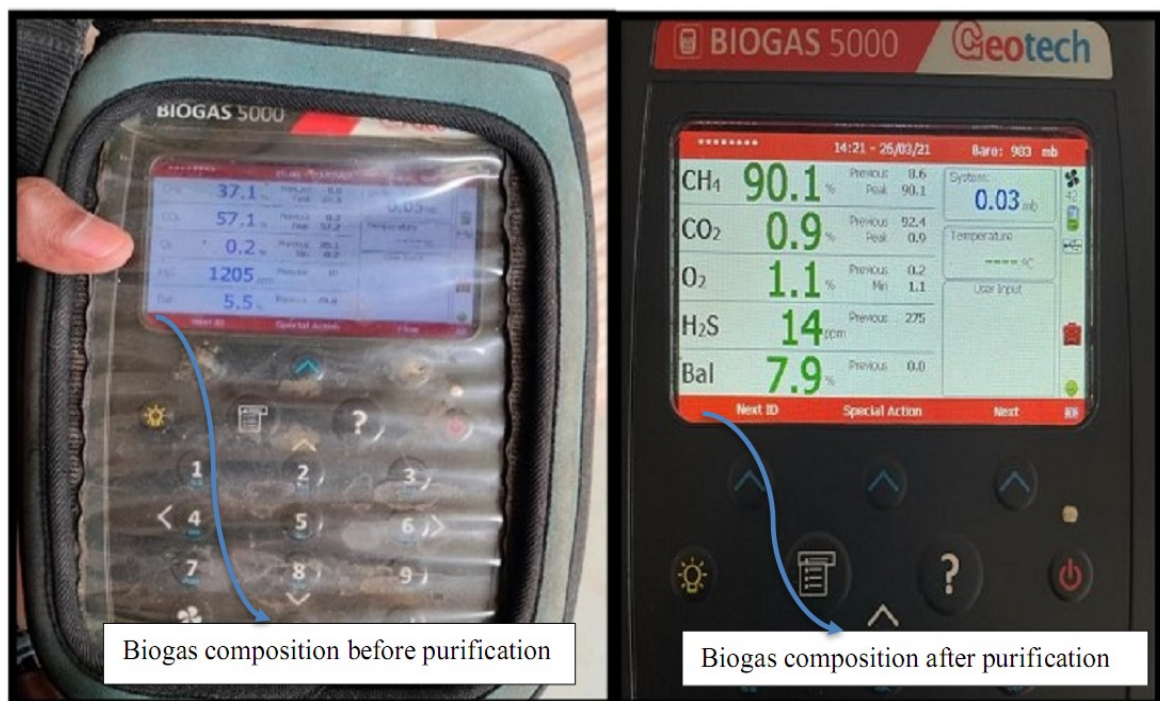
Figure 4.6: Portable biogas 5000 analyzer
