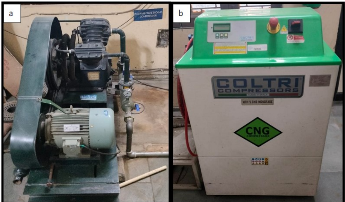
Figure 4.7: Biogas compressor (a) low compressor up to 10-12 bar (b) high compressor up to 200-250 bars
