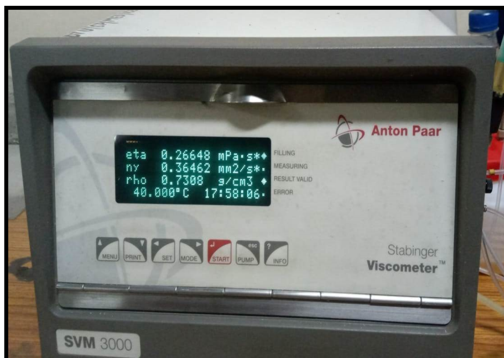
Figure 5.2: Viscometer- fuel density tester
