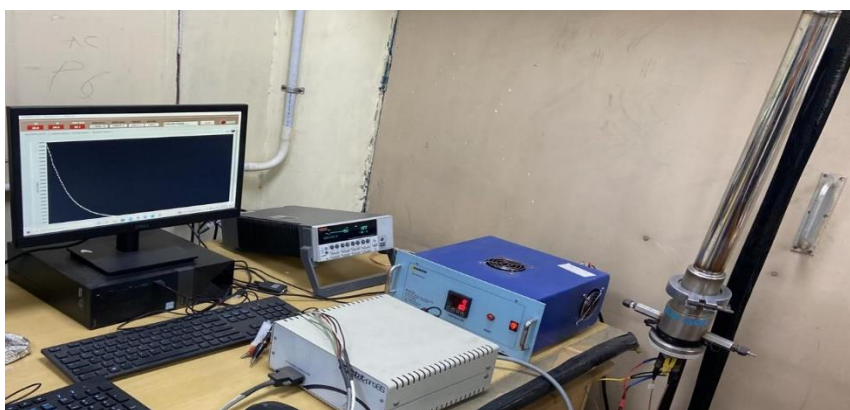
Figure 2.7. Source Measurement Unit (SMU) for electrical conductivity Measurement.
