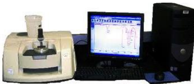
Figure 2.5 FTIR instrument for Vibration Analysis.
