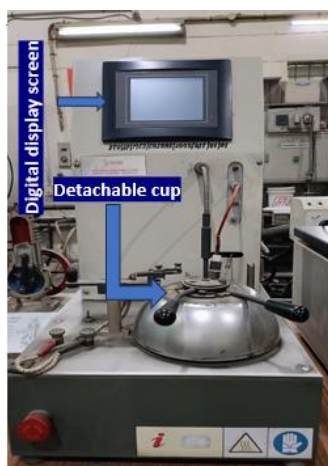
Plate 3.5: Flash point apparatus
