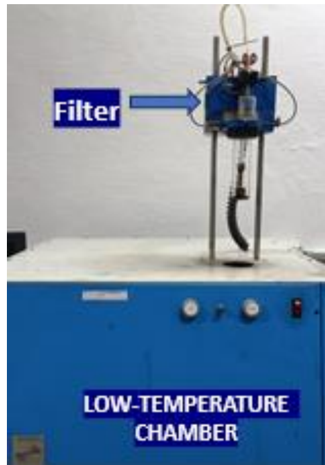
Plate 3.7: Cold flow plugging point apparatus
