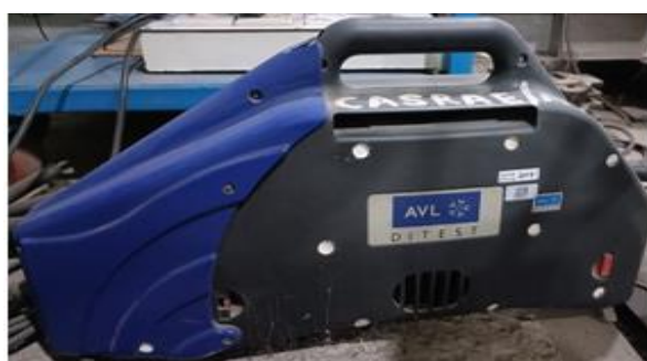
Plate 3.14: AVL Exhaust gas analyzer
