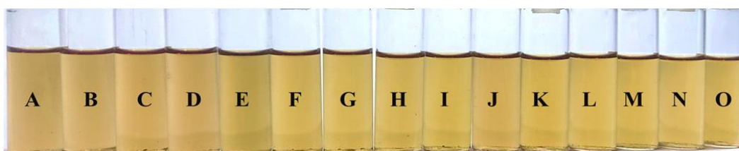
Figure 4.3. The observed colour-change upon addition of 1.0 equivalent tetrabutylammonium salts of different anions into a solution of Co-(1-5) in acetonitrile. From left to right; A =Without anion, B = \text{CN}^- , C = \text{F}^- , D = \text{CH}_3\text{COO}^- , E = \text{Cl}^- , F = \text{Br}^- , G = \text{I}^- , H = \text{NO}_3^- , I = \text{H}_2\text{PO}_4^- , J = \text{PF}_6^- , K = \text{AsO}_3^{3-} , L = \text{AsO}_4^{3-} , M = \text{ClO}_4^- , N = \text{S}^{2-} , O = \text{HS}^- ,
