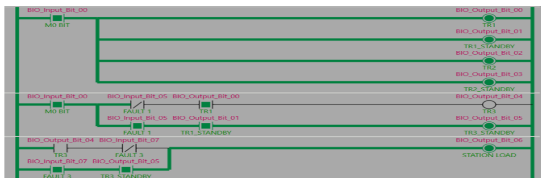
Figure 5.24. Ladder logic program of PLC in case of faults (when Aux T-1, Aux T-2, Aux T-3 is standby)
