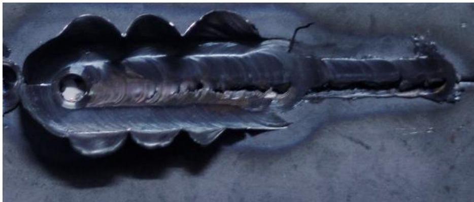
Figure 4.9: Thinning of material because of excessive flash
