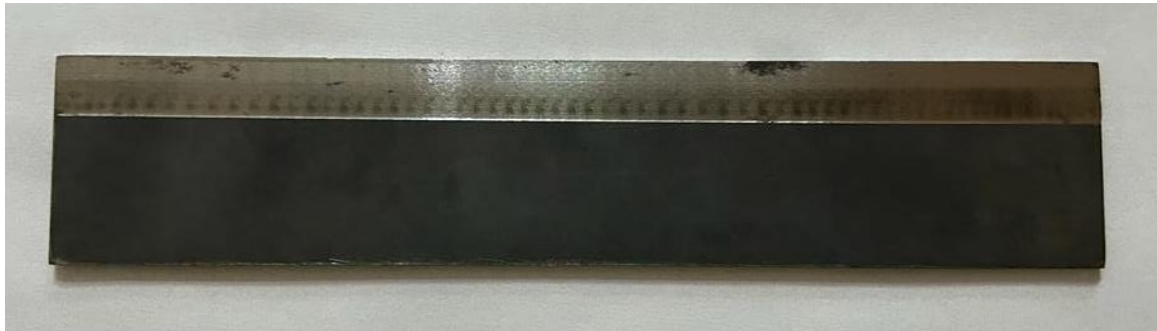
Figure 4.11: Plate with the edges cleaned and ready for welding
