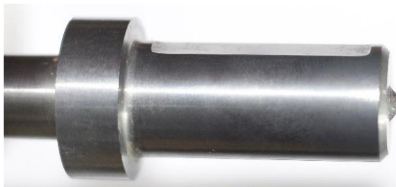
Figure 4.3: Wearing of tool pin when cylindrical pin profile was used.
