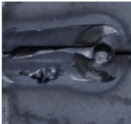
Figure 4.7: Shoulder void defect due to insufficient tool tilt
