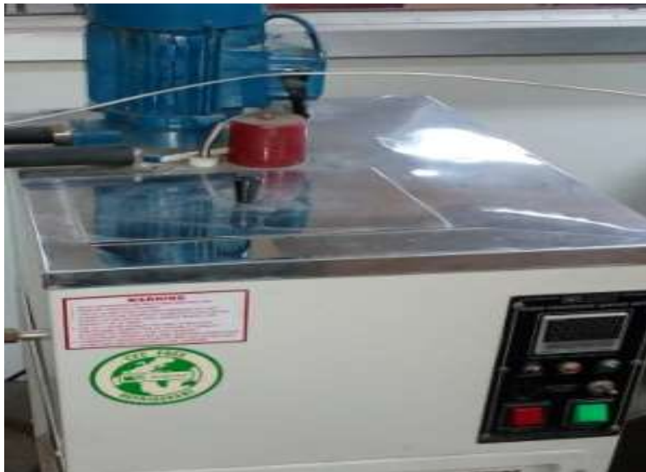
Fig.13: Chiller for cooling the electromagnetic coil
