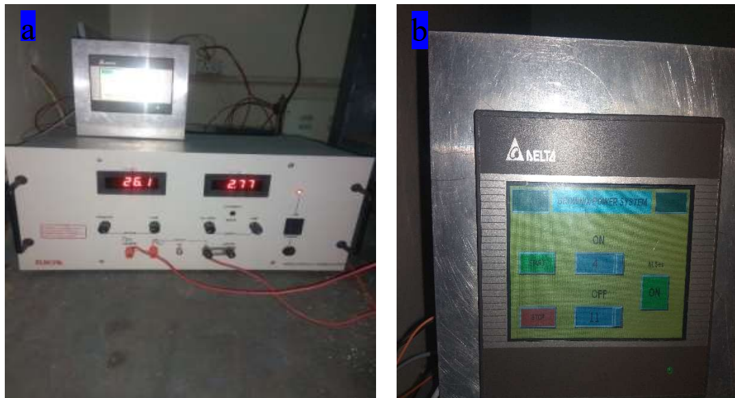
Fig.15: (a) Pulse DC power supply (b) HMI unit for adjusting pulse ON/pulse OFF value
