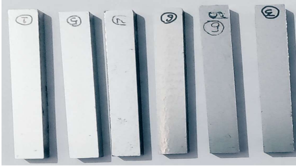
Fig.24: Finished EN-31 work-piece using pulse DC power supply at 2.5A, 50 mm/min, 1.5 mm and 500 rpm
