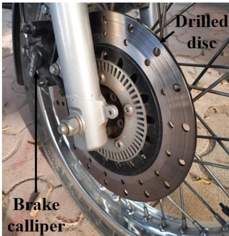
Fig. 8.1 Two-wheeler brake disc assembly
