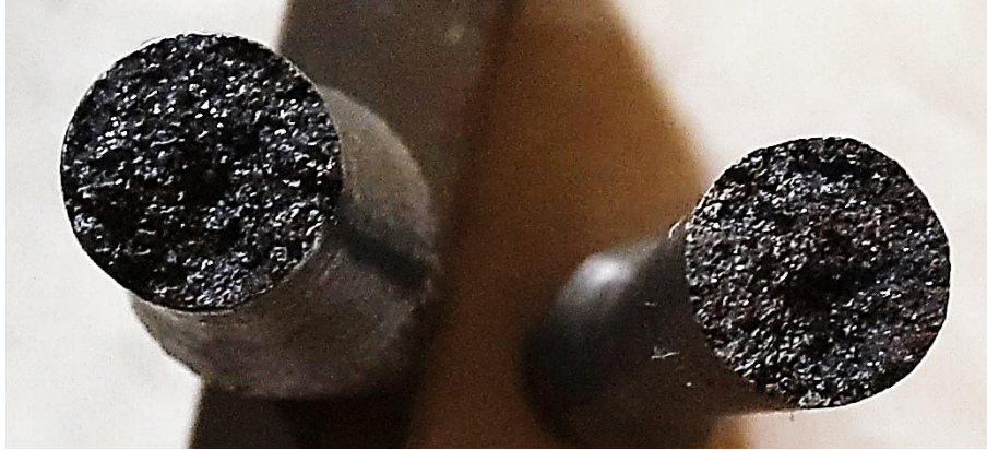
Fig. 4.12 Fracture surface of tensile tested specimen
