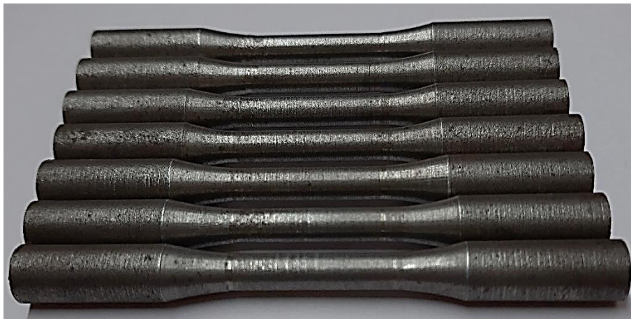
Fig. 5.1 Tensile test specimens for evaluation of J - C parameters
