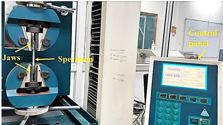
Fig. 4.11 Tensile test setup on universal testing machine (Tenius Olsen)
