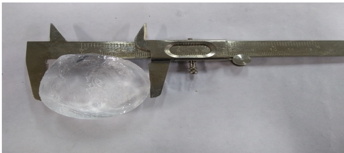
Fig 6 Swollen hydrogel (diameter 5.09cm, thickness 2.56cm)
