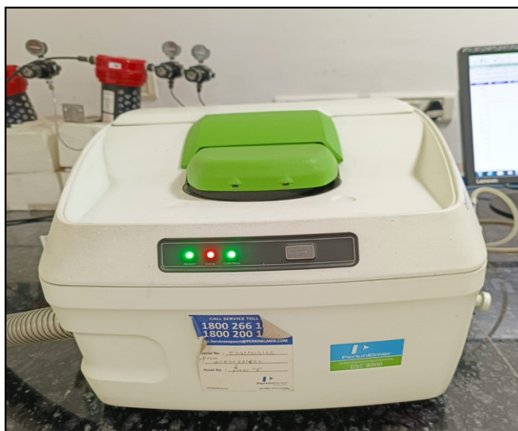
Figure 2.8: Differential scanning calorimeter (DSC 8000, Perkin Elmer) used to determine phase change characteristics
