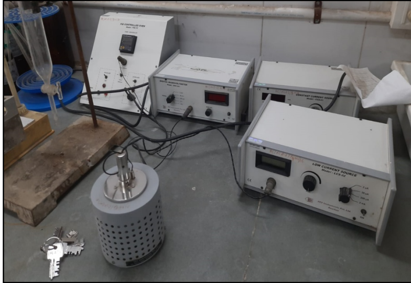
Figure 2.18: Electrical Resistivity Four point probe setup
