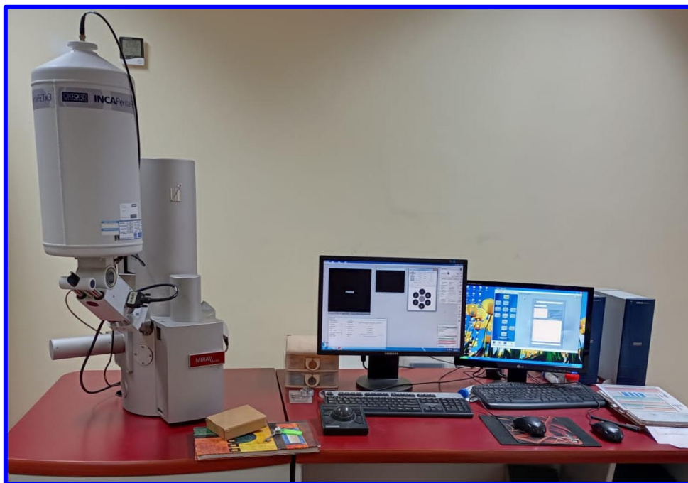
Figure 2.7: MIRA-II TESCAN Field emission scanning electron microscopy setup.
