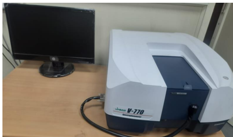
Figure 2.8: UV-Visible spectrophotometer of Jasco company with Model V-770 setup.
