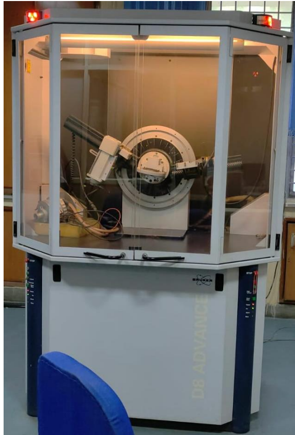
Figure 2.4. XRD machine of Bruker company with Model-D8-advance setup.
