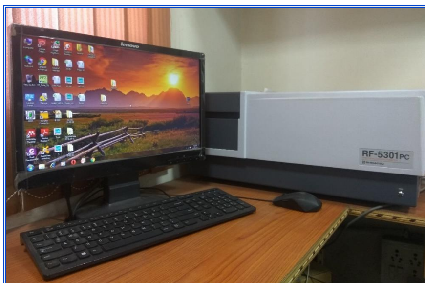
Fig. 2.11: Shimadzu, RF-5301PC spectrofluorometer connected with computer.
