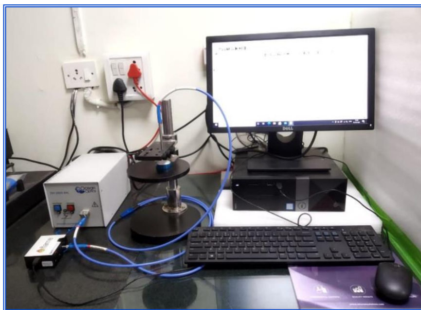
Fig. 2.14: TDPL characterization setup with ocean Optics spectrofluorophotometer
