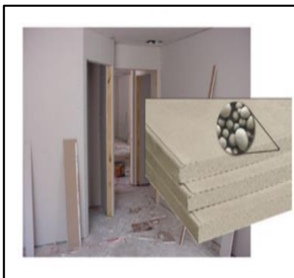
Figure 12 PCM enhanced gypsum boards [80]
