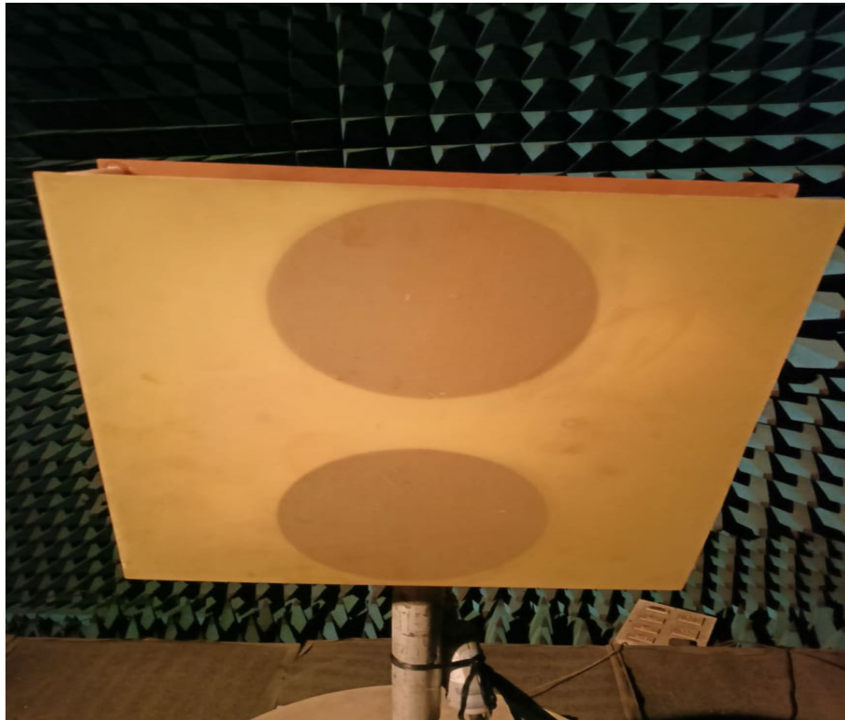
Fig. 4.18 Antenna design-I for gain measurement
