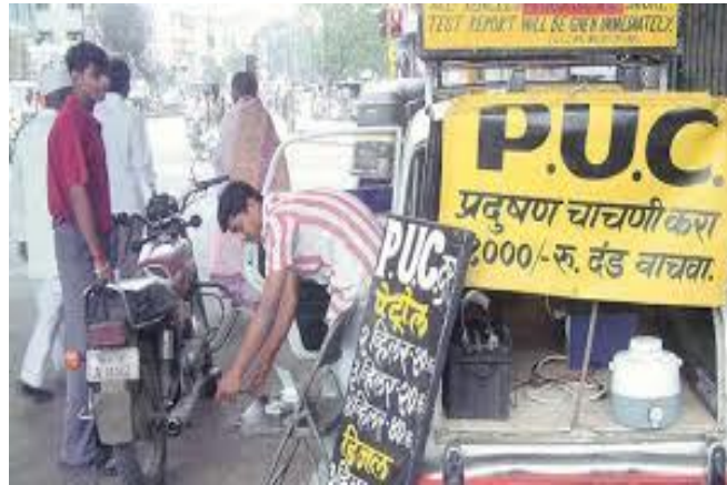
Fig 3.4– A 2-Wheeler been tested using the 2- gas analyzer at an authorized PUC test dealer in Delhi
