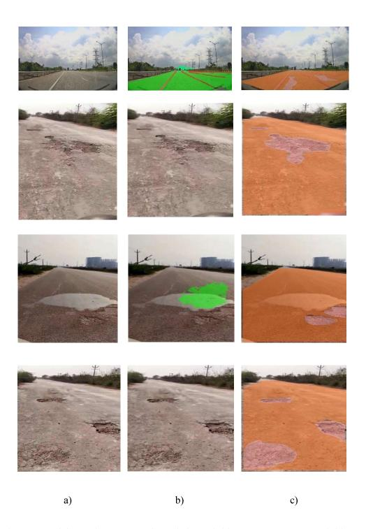
Fig. 5.1 Model Results a) Ground Truth b) HybridNets c) YOLOv7. HybridNets is incapable of performing pothole detection. Also, it is only capable of identifying smooth roads, as in case1 and fails to detect roads that are improper or slightly damaged in rest of the cases. YOLOv7 detects the roads in either of the cases.
