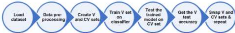
Fig 5.2 Flow chart of the training and testing process.
