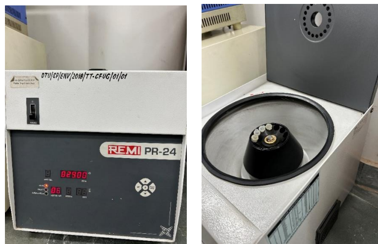
Fig 3.6 Sample preparation for spectrophotometer by using centrifuge machine
