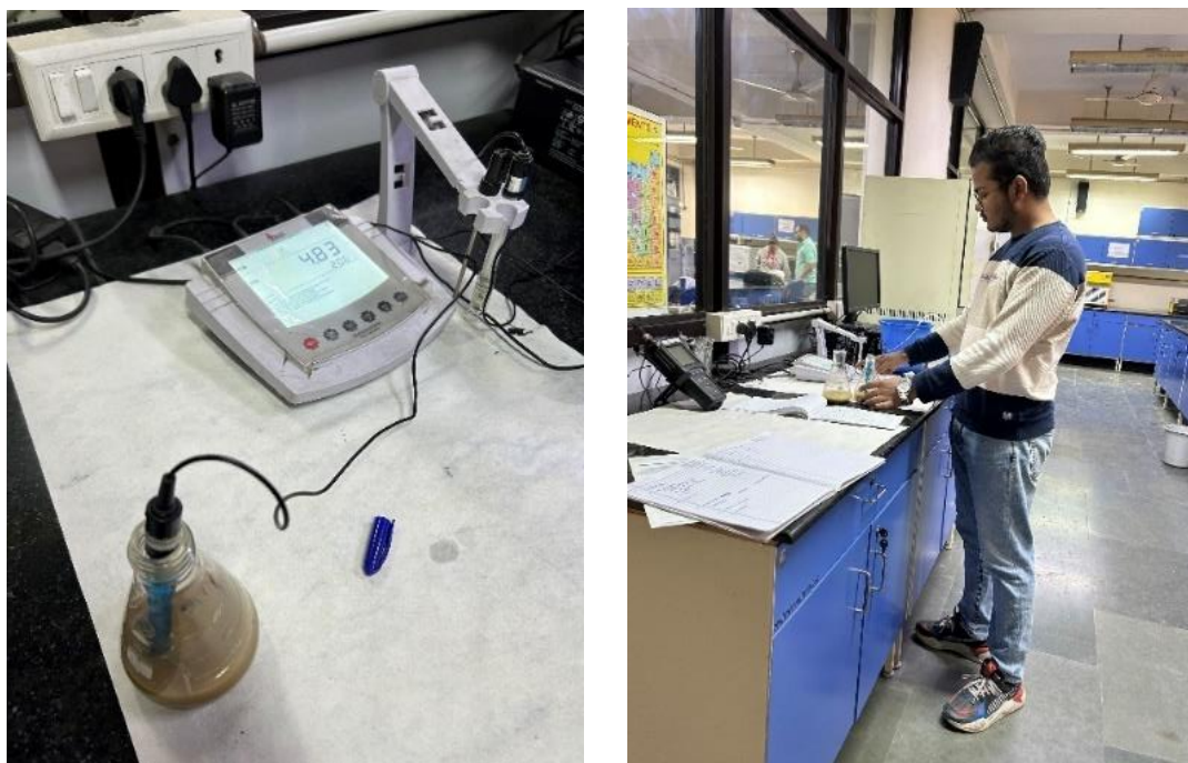
Fig 3.7 Use of Water quality Multiparameter to find parameters like pH, Conductivity, TDS etc.
