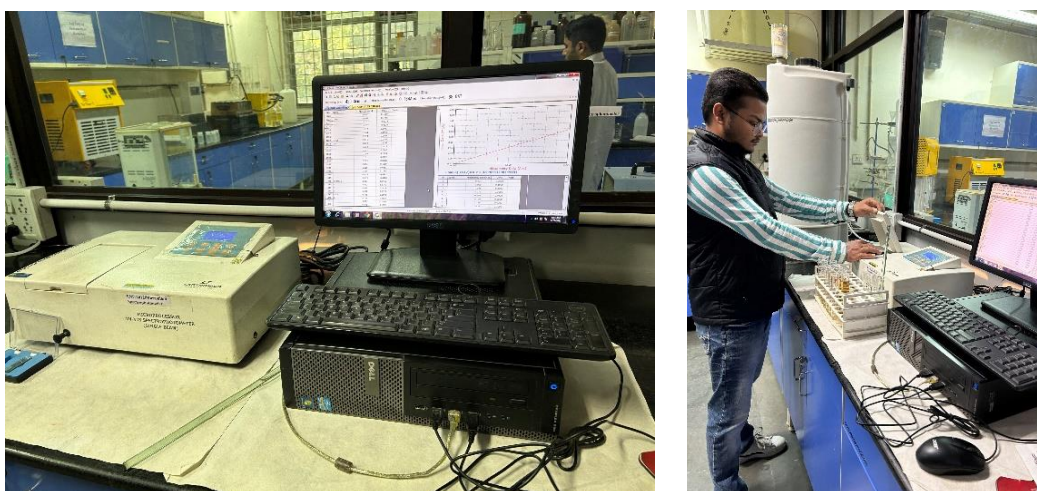
Fig 3.9 Use of Spectrophotometer for finding content of Sulphate Phosphate and Nitrate
