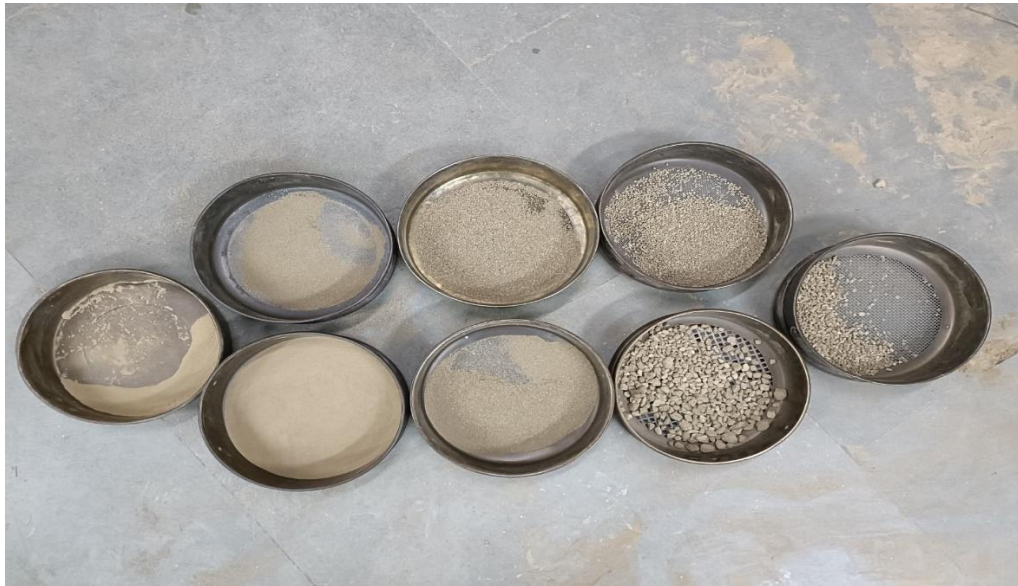
Fig. 3.2 Sieve analysis according to IS code.
