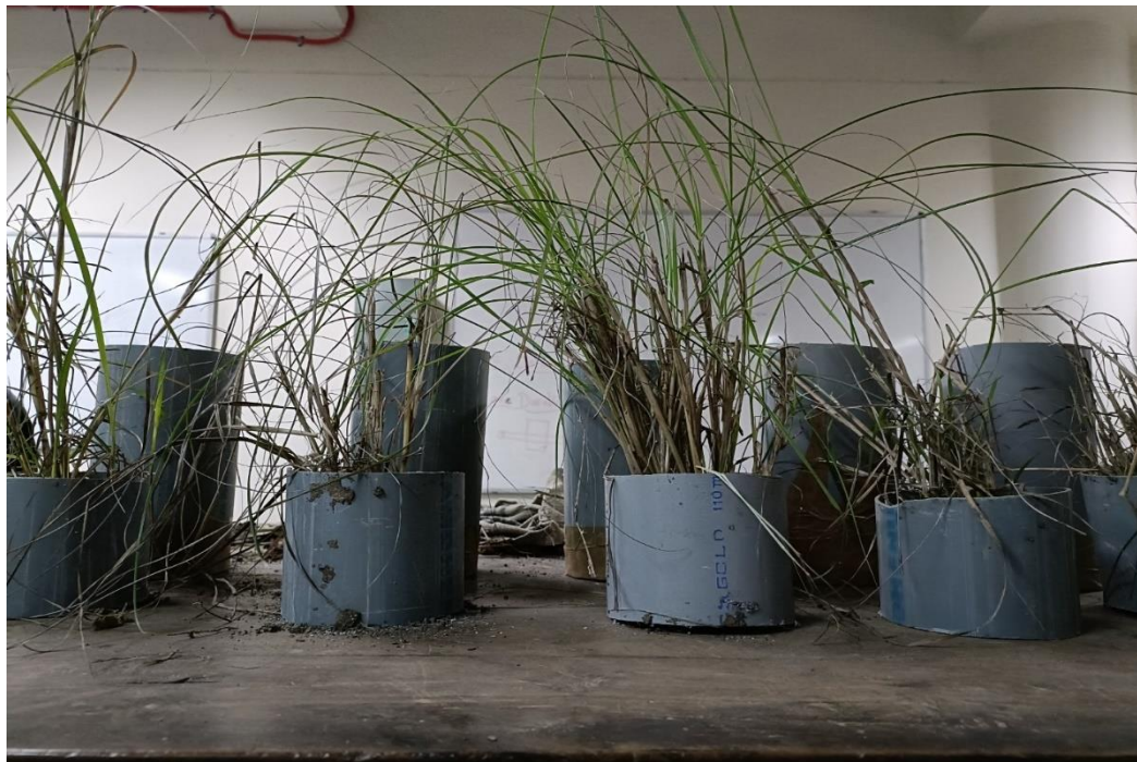
Fig. 3.3 Direct shear sample of rooted soil cut 10cm from the top
