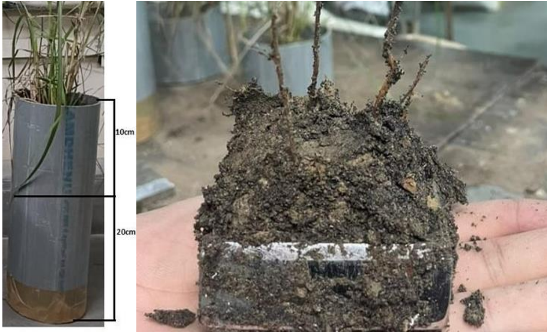
Fig. 3.4 (a) Layout of planted PVC; and (b) Sample of the direct shear test.
