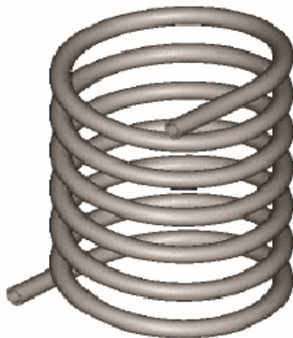
“Figure 1.8: Helical coil type pipe”
