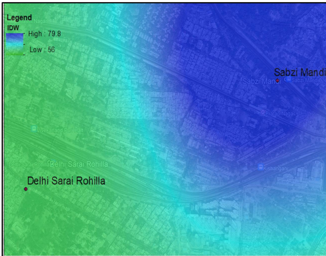
Figure 4.5. Noise mapping showing variation of noise levels from 10 pm to 6am
