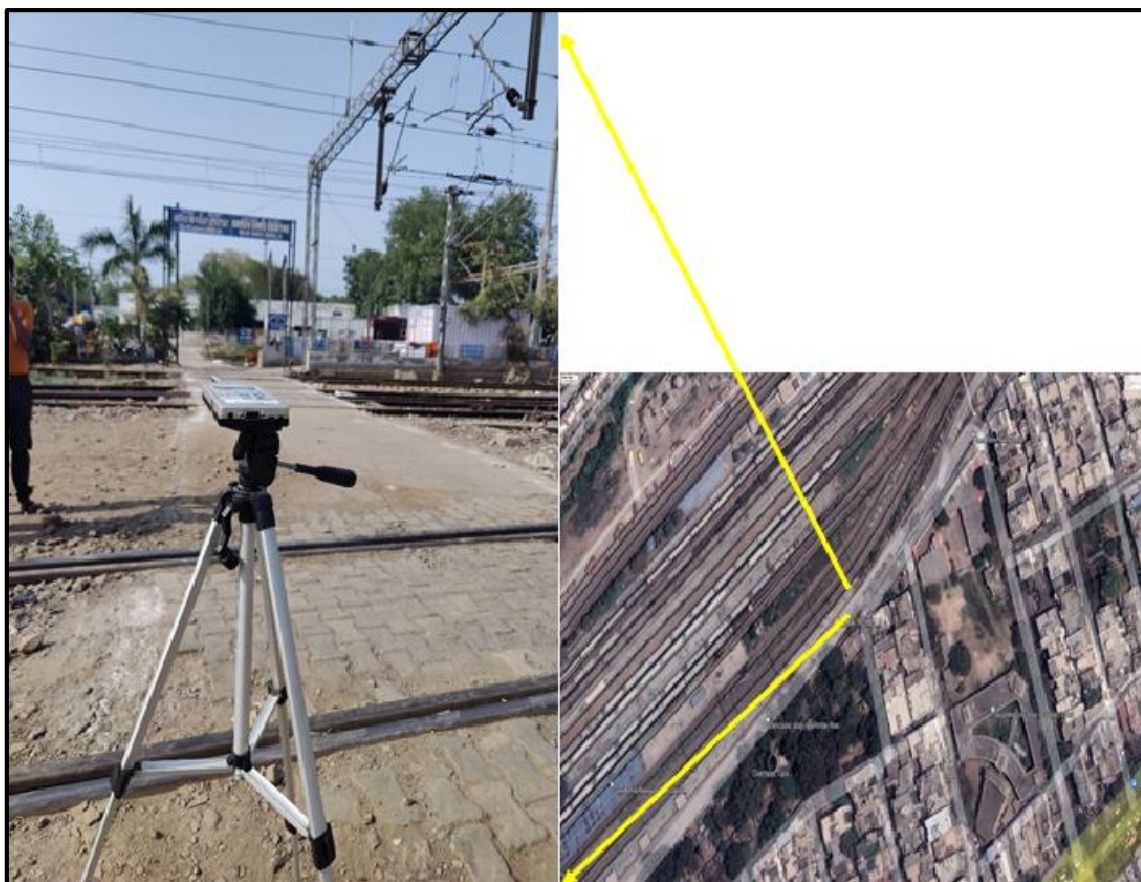
Figure 3.4. Noise monitoring at Sarai Rohilla Railway Station
