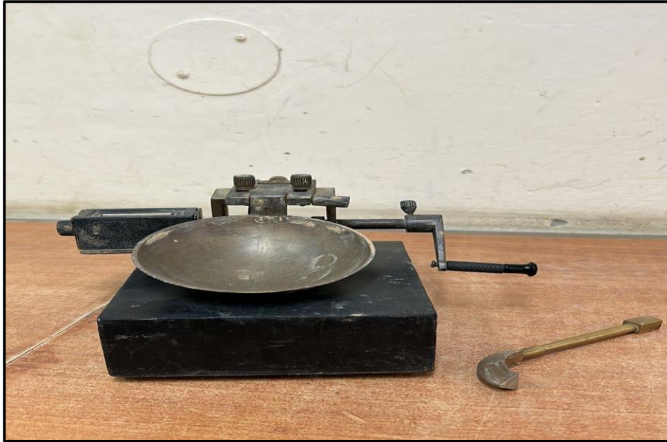
Fig 4.4: Shows Casagrande's apparatus for liquid limit determination
