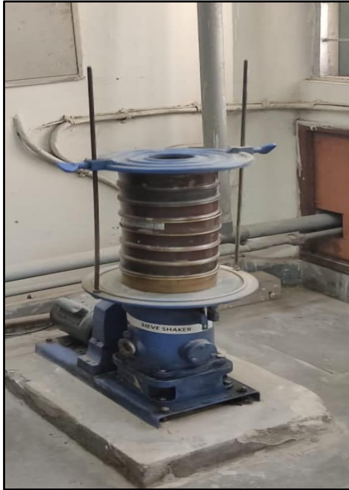
Fig 4.3: Sieve arrangement placed on a sieve shaker
