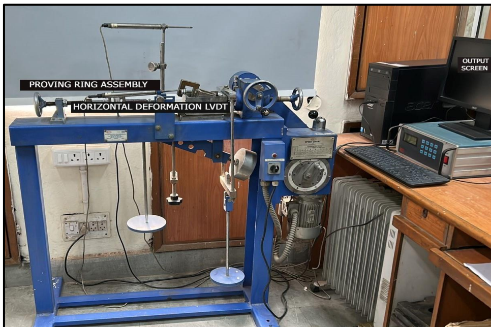
Fig 4.7: Shows the Direct Shear Test Assembly
