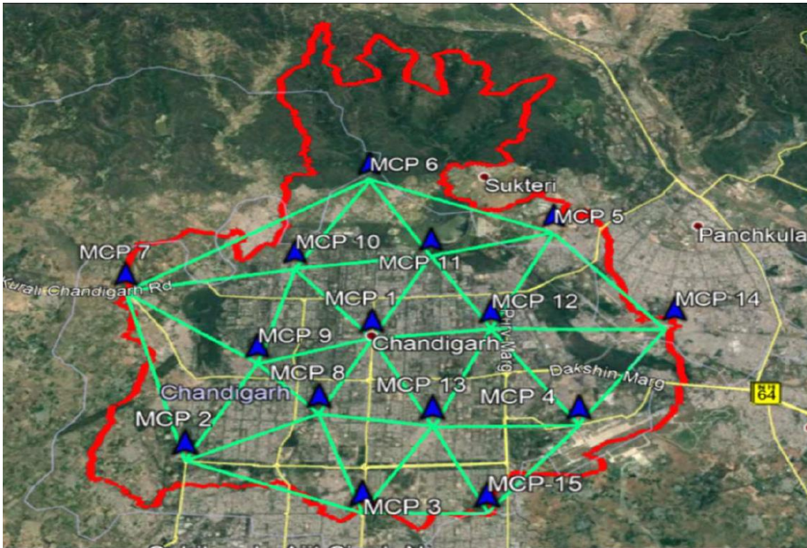
Figure 38: Master Control Network
