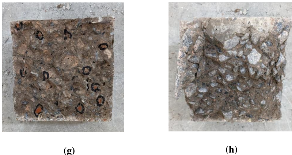
Fig. 4.8 (a);(b);(c);(d) represents compression test of samples CM, 20RAC0, 10RAC10, 0RAC20 respectively; (e) Rebound Hammer test on CM; (f) Crushed 20RAC0 sample indicating CDCA particles; (g) Crushed 10RAC10 sample indicating CDCA particles; (h) Crushed 0RAC20 sample
