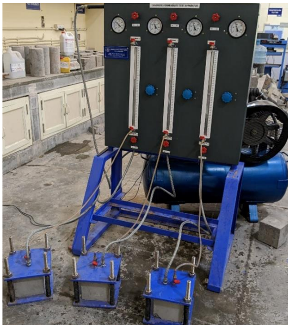
Fig. 3.6 Concrete Permeability testing equipment
