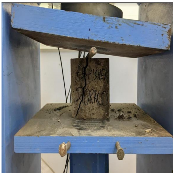
Fig. 3.7 Shearing of specimens to achieve water penetration depth.
