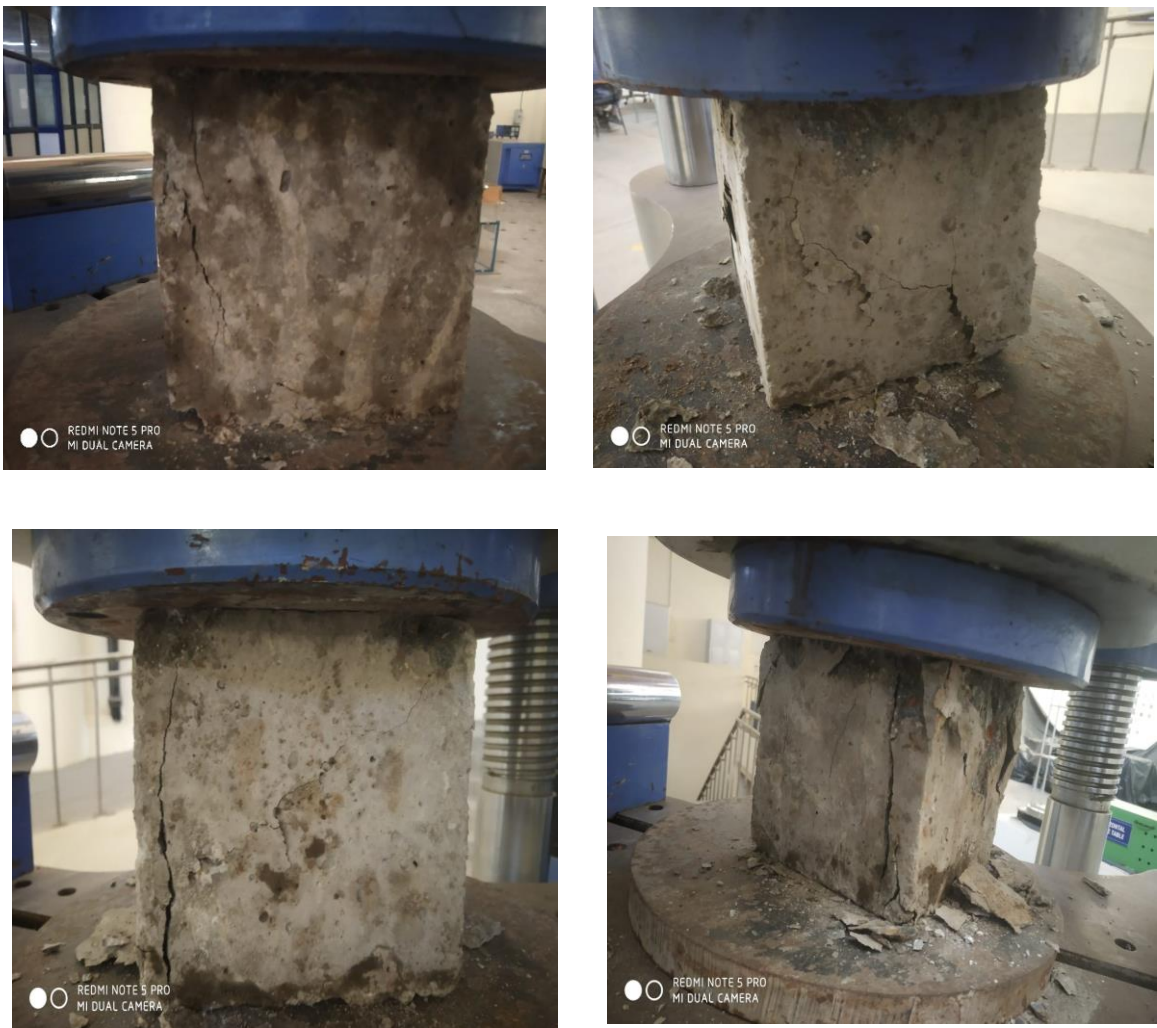
Fig 4.2 Different Types of Cracks
