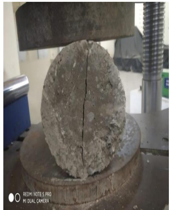
Fig 4.8 Crack Formation on the Cylinder
