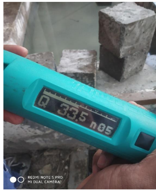
Fig 4.15. Rebound hammer Reading 5
