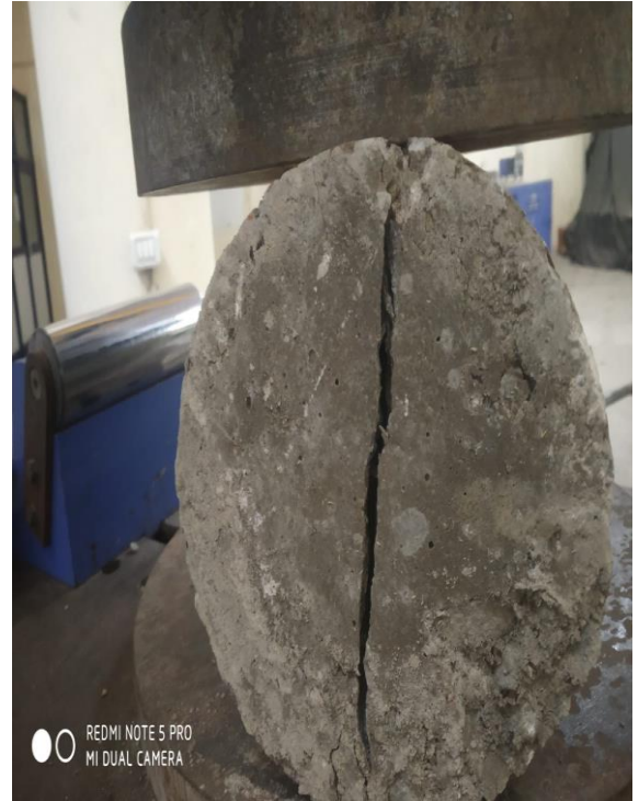
Fig 4.10 Large Crack Developed on the Cylinder
