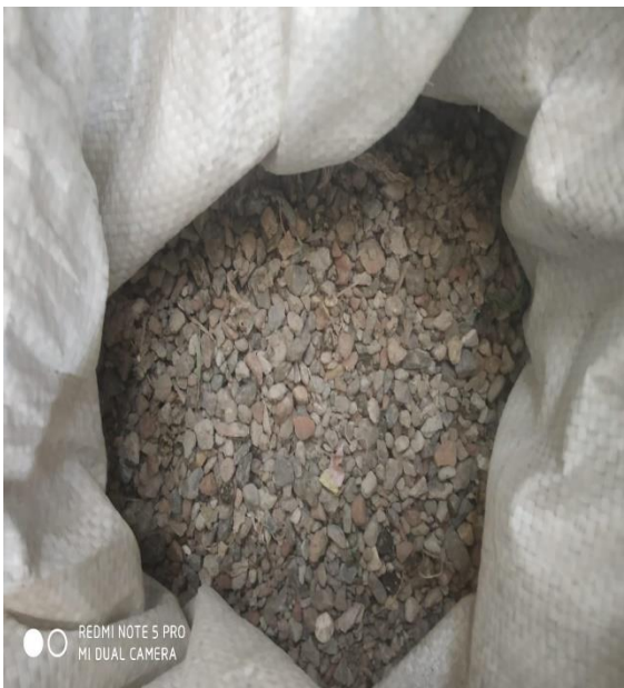
Fig 3.5 Demolition Waste of 10mm
