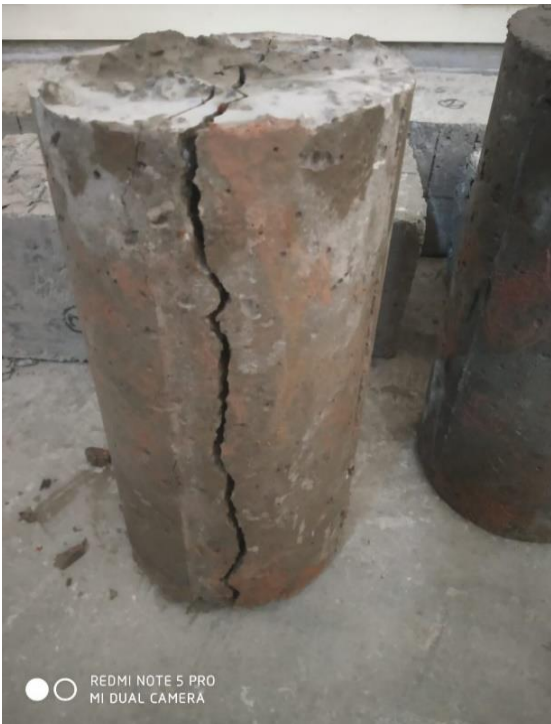
Fig 4.11 Crack Seen on Length Wise
