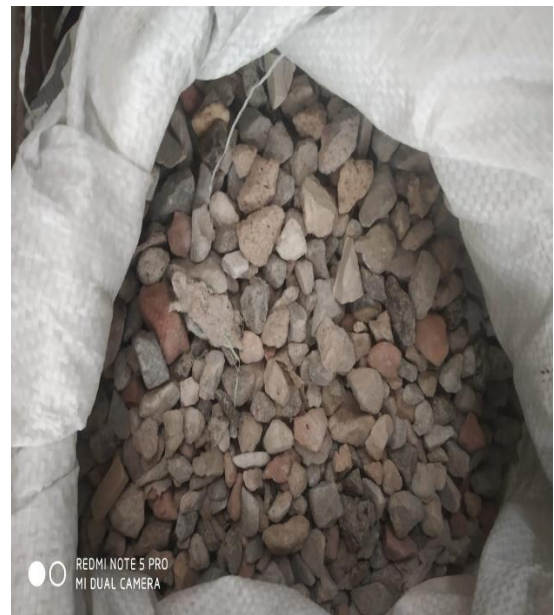
Fig 3.6 Demolition Waste of 20mm
