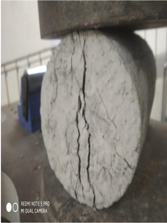
Fig 4.9 Formation of Various Crack on the Cylinder
