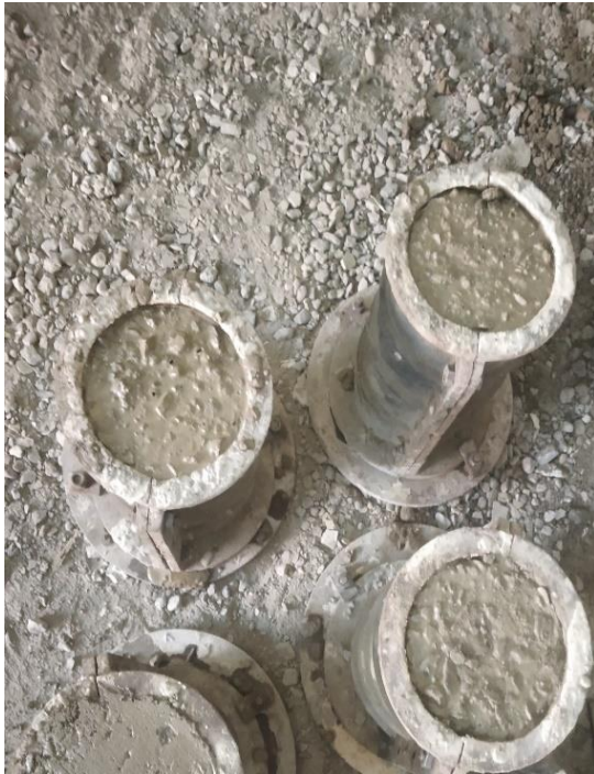
Fig 4.5 Casting of Cylinder
