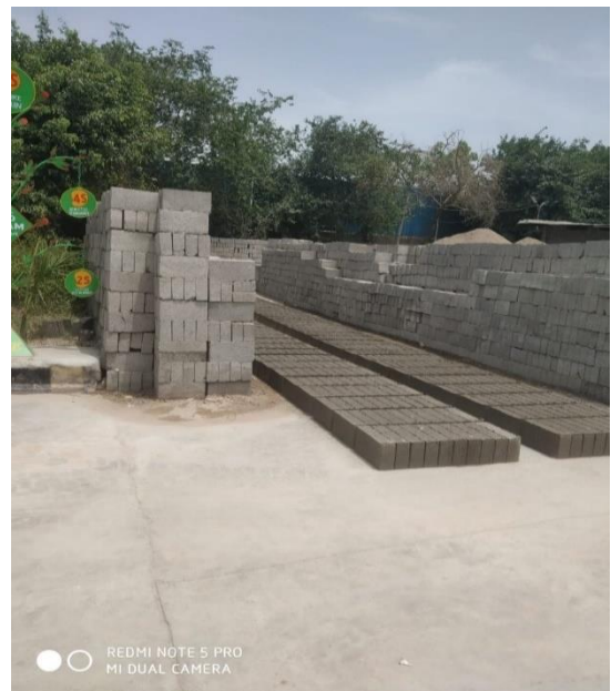
Fig 3.8 Made building blocks using Demolition waste
