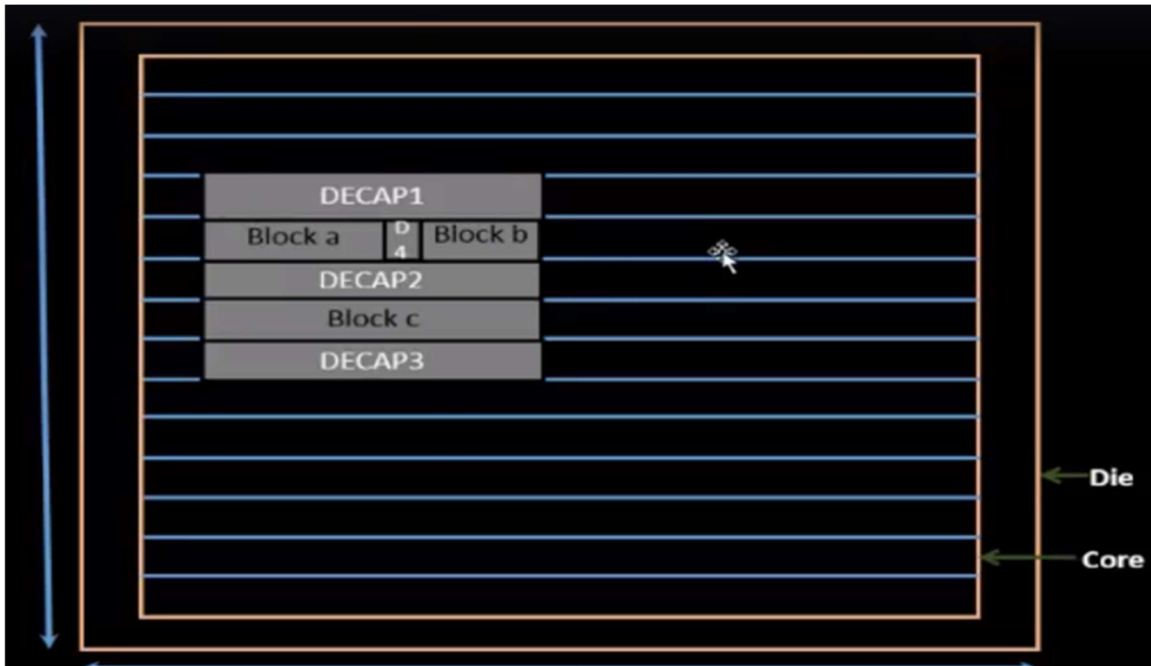
Fig 2.7(c) Placement of decoupling capacitors on IC
