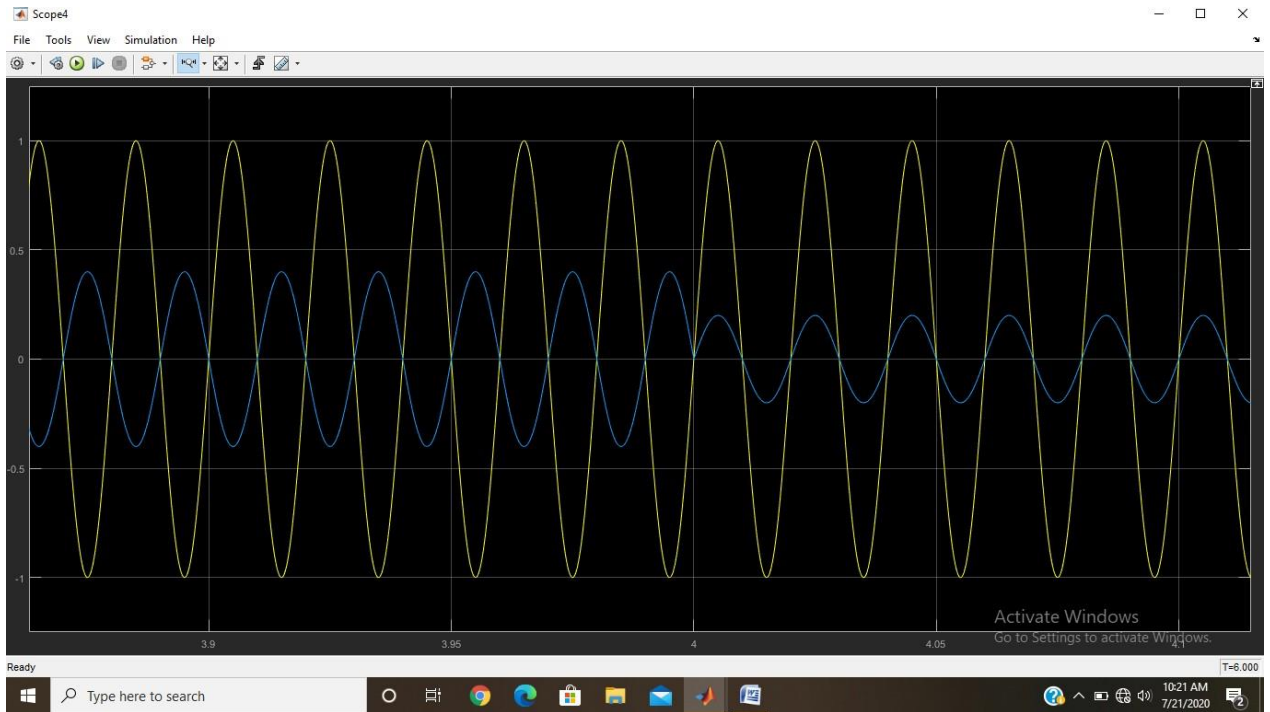
Fig. 4.14 G2V (Grid-to-Vehicle) state, both the voltage and current are synchronized
