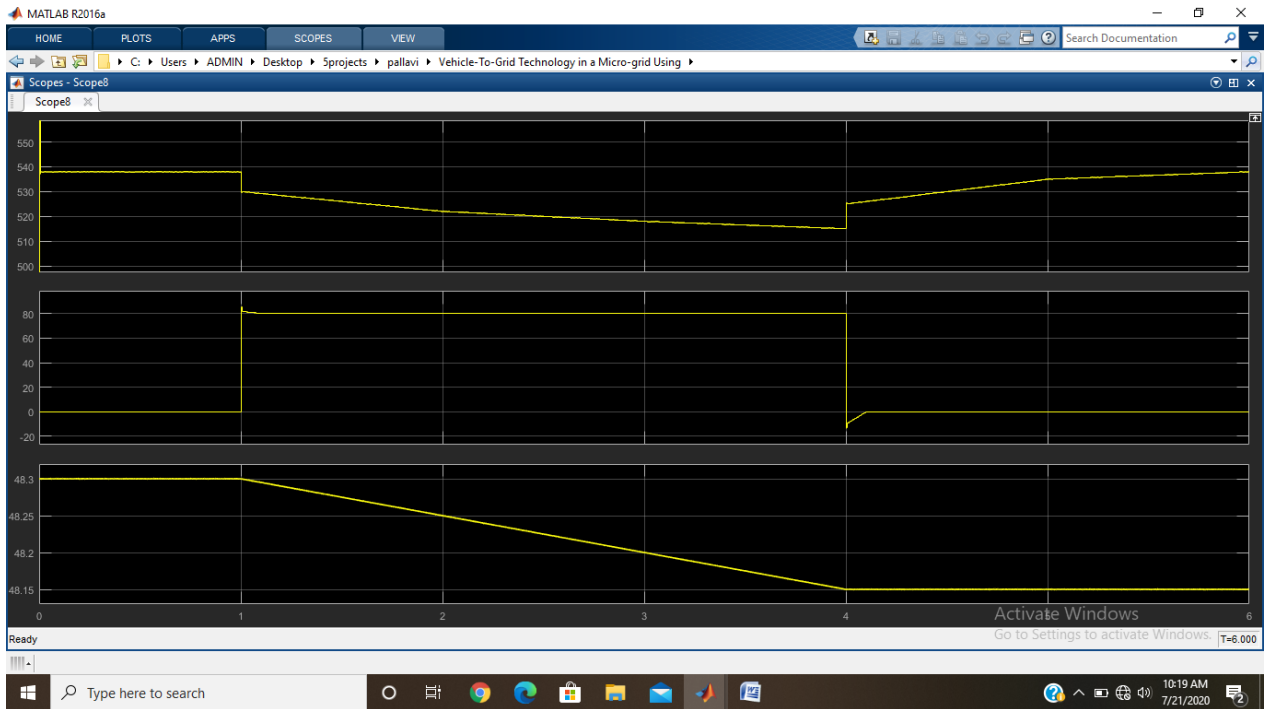
Fig. 4.2 Voltage, current, and SOC of EV1 battery during V2G operation.
