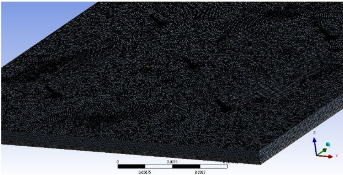
Fig. 3.7. Meshing of inclined hexagonal 5 hex-jet heat sink, E60
