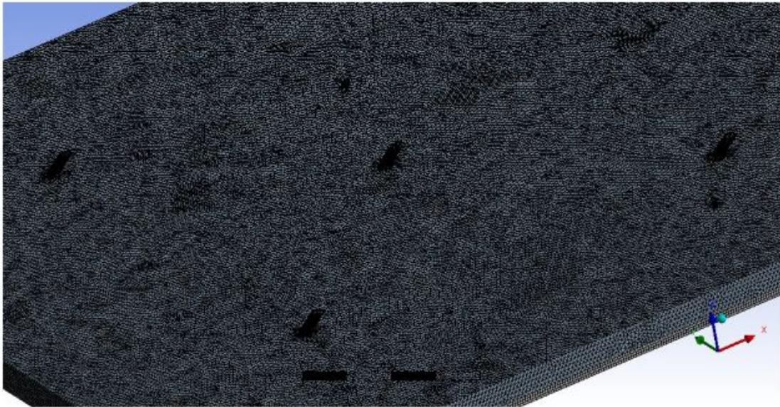
Fig. 3.17 Meshing of inclined hexagonal 5 hex-jets heat sink, E80
