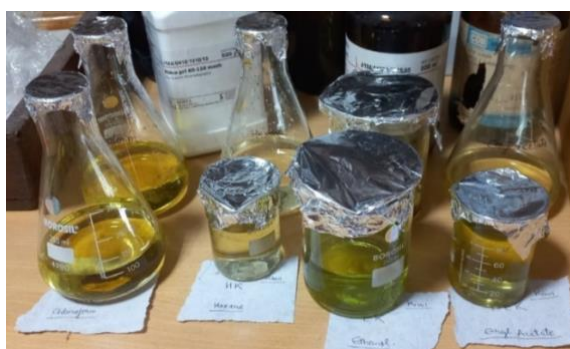
Figure 22 – Powdered Kiwi peels put in 4 different solvents– Chloroform, Ethanol, Hexane, and Ethyl acetate
