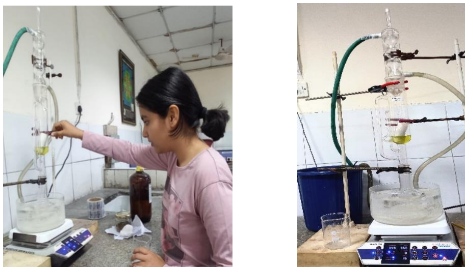
Figure 23 – Soxhlet Apparatus set-up
