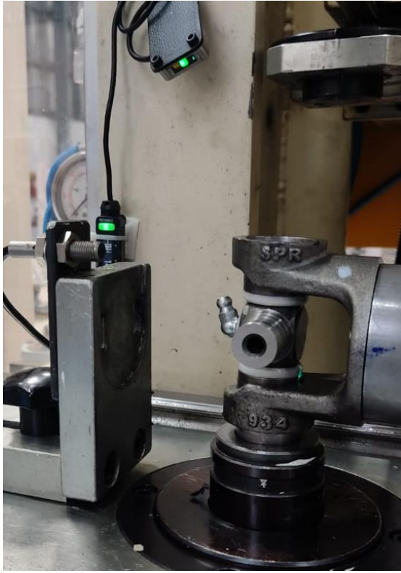
Figure 29 Alignment of grease nipple in SY
