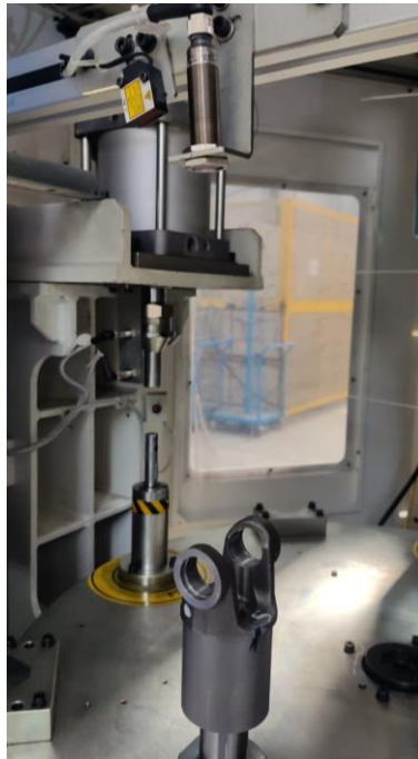
Figure 27 Poka yoke for O ring missing
