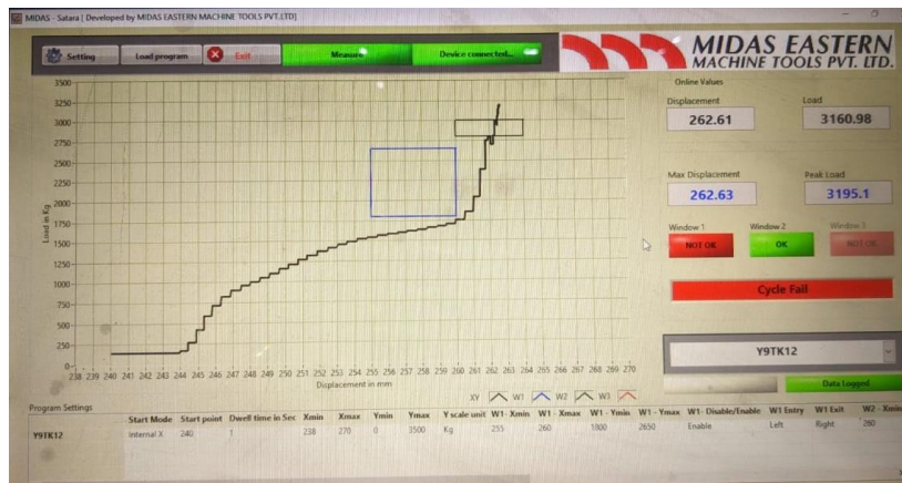
Figure 22 Graph passing out of set window/Rejected part
