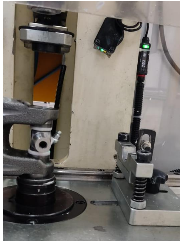
Figure 30 Alignment of grease nipple in FY
