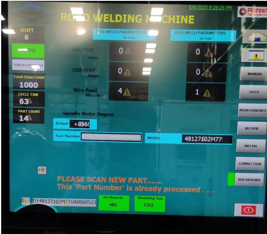
Figure 24 Program display for not repetition of same shaft to weld
