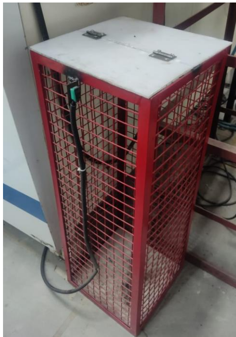
Figure 25 Rejection bin for MIG welding
