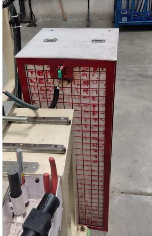
Figure 35 Rejection bin for part not able to be corrected
