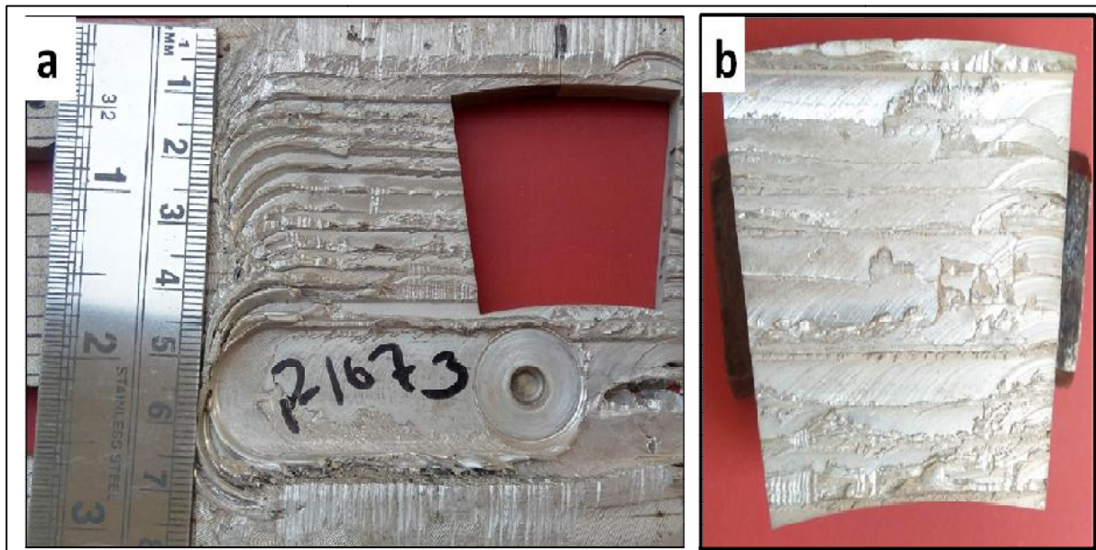
Figure 4.32 (a) Pad shape piece cut from the processed zone (b) Fabricated FSPed cast AS21A alloy sector shape pad
