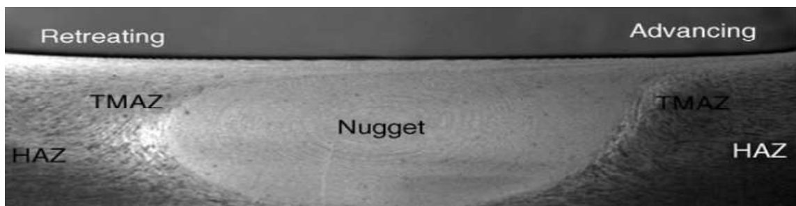
Figure 1.9 Different zones in the cross-section of FSPed 7075Al-T651 [49].
