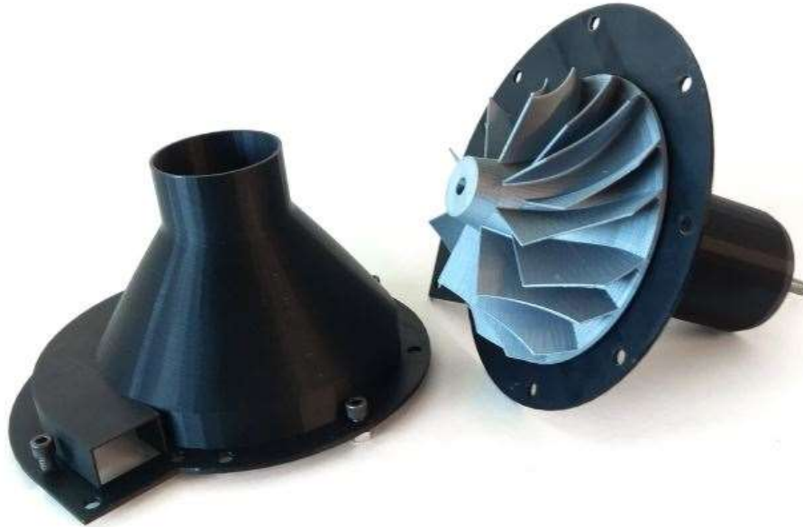
Figure 1.8: Turbine with hub casing [32]
