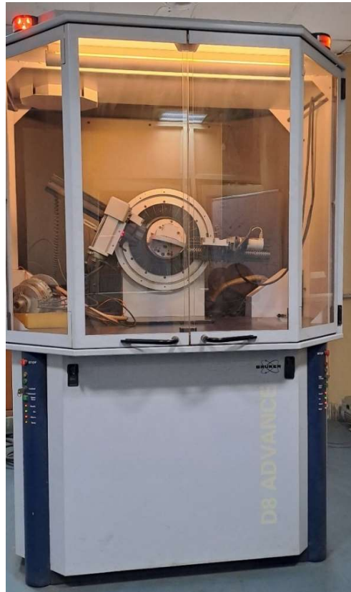
Figure 3.14: Bruker advanced D8 XRD testing machine
